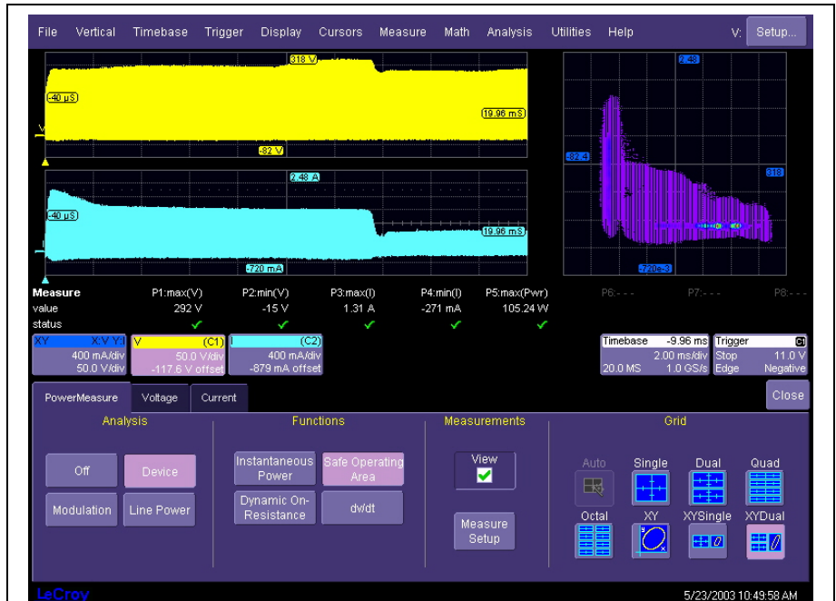
Figure 4 The SOA plot for power supply startup shows a more severe operational range of voltage, current and power.
